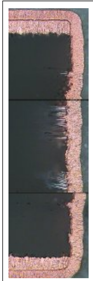
Figure 13: Microsection of 10:1 aspect ratio panel plated with modified pulse parameters
