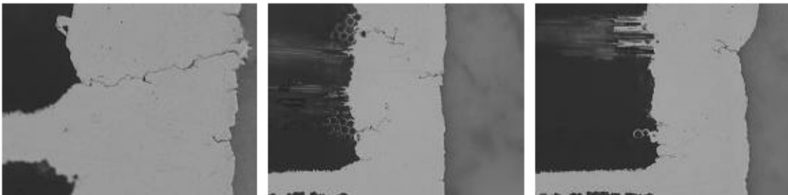
Fig. 9: Cracks which can be found at approx. 1 % increase in warm state resistance (from the same experiment as shown in Fig. 6).
