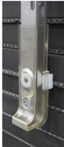
Figure 5: High performance clamp for thin copper foil and thin panel capability.
