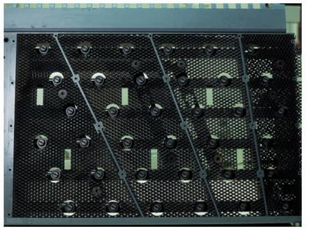
Figure 4: Segmented anode unit to ensure optimum surface distribution.
