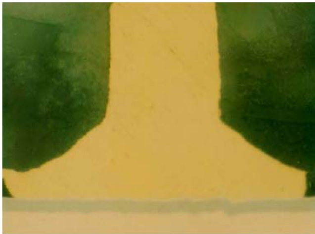
Fig. 15 Image of gold ball bond on Ni/Pd/Au following 2000 hours heat conditioning (150°C)
