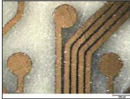
Fig. 8 Pads and trenches after laser ablation, and after complete circuitization.
