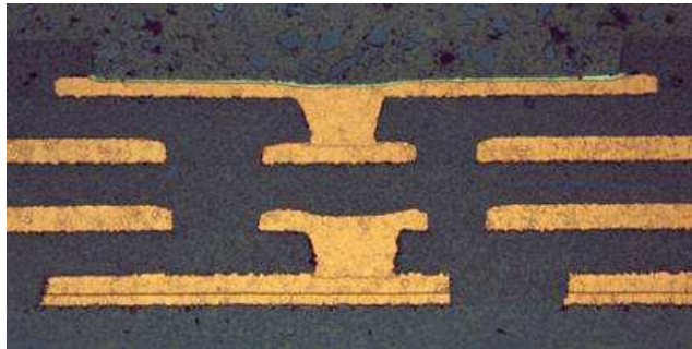
Figure 2 – IC Substrate with Copper Filled Build-Up Layers.
