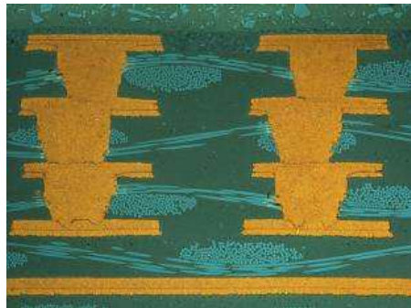
Figure 3 – Stacked Filled Blind Micro Vias
