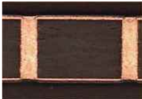
Figure 12 - Copper Filled Through Hole Panel Thickness 0.4 mm Hole Diameter 100 \mu\text{m} . Surface Plated Copper 19 \mu\text{m} .
