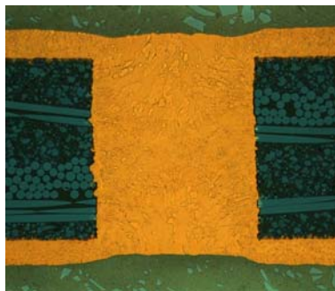
Figure 10 - Filled Through Hole 120 \mu\text{m} thick, 100 \mu\text{m} Diameter with Total Surface Plated Copper 13 \mu\text{m} .
