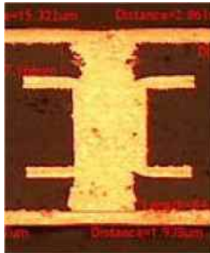
Figure 11 - Core filled with electrolytic copper followed by filled BMV with minimum surface plated copper.
