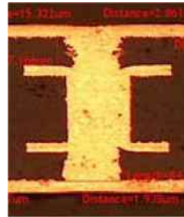
Figure 16. Core filled with electrolytic copper followed by filled BMV with minimum surface plated copper.
