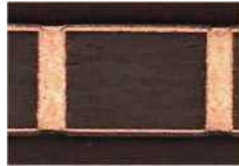
Figure 17. Copper filled via thickness 0.4 mm diameter 100 \mu\text{m} . Surface plated copper 19 \mu\text{m} , laminate copper foil 35 \mu\text{m} .
