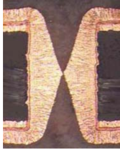
Figure 9. Exaggerated copper plating in through via
