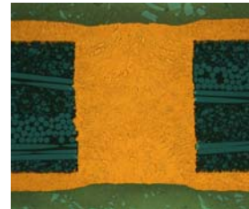
Figure 11. Filled through hole 120 µm thick, 100 µm diameter with total surface plated copper 13 µm.
