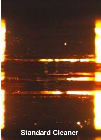
Pictures 11-12 – Backlights showing better coverage with Improved Flex Cleaner
