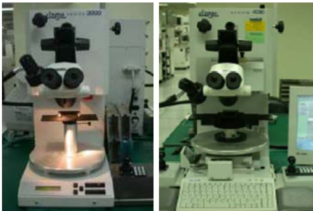
Fig. 3 Dage Series 3000 Wire Pull Tester (left) and Dage 4000 Solder Ball Shear Tester (right)
