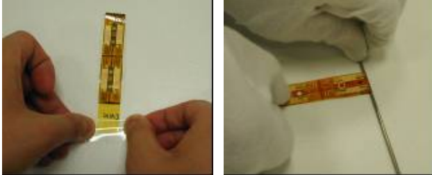
Fig 16 Securing the flex circuit sample (left) and performing the 2-mm wire pull/bend test (right)
