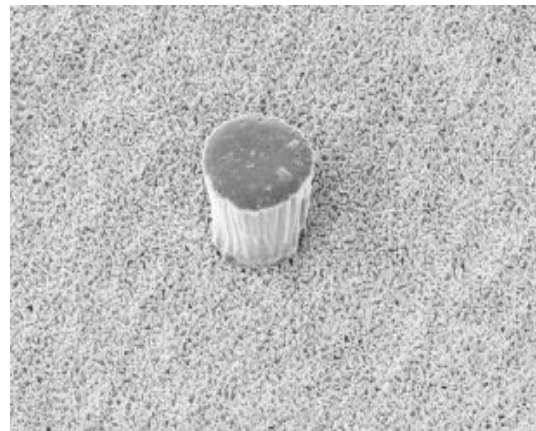
Fig 14 – SEM Image of Single 75- \mu\text{m} Column
