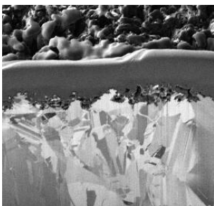
Figure 2. Typical Oxide Alternative Structure
