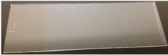
Figure 1: Glass panel with film deposited from water based coating formulation VitroCoat GI W.
