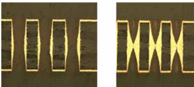
Figure 9: Effect of ferric ions on the X-formation: left 1.0 g/l right 0.5 g/l ferric
