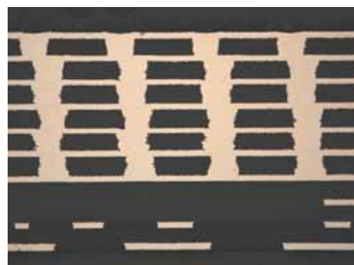
Figure 7: Filled stacked BMV, also called "Any Layer".
