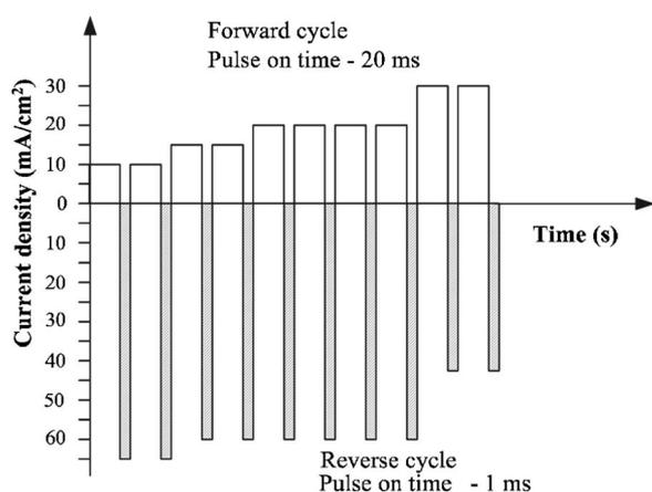
**Figure 3.** Variation in forward and reverse current density with electroplating time.
