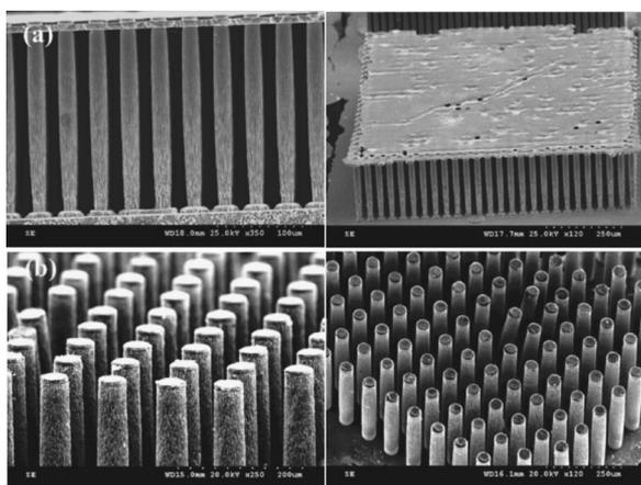
**Figure 4.** High aspect ratio through-wafer copper interconnects after the dissolution of silicon. (a) Diameter 15 μm, pitch size 35 μm, aspect ratio 15. (b) Diameter 30 μm, pitch size 80 μm, aspect ratio-12.
