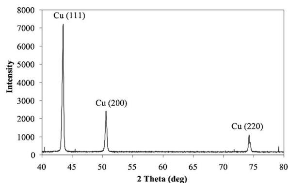
**Figure 5.** XRD analysis showing  $\langle 100 \rangle$  crystal orientation of copper electroplated interconnects.
