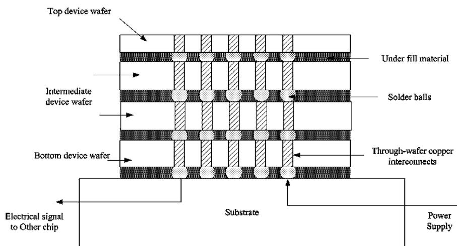
Figure 1. Schematic representation of 3-D wafer stacked device.
