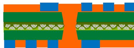
**Figure 5:** Pattern plating for fine line application: the challenge of within unit distribution and inclusion free filling
