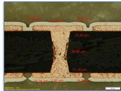
**Figure 7:** Example of filled 0.15mm thick through hole
