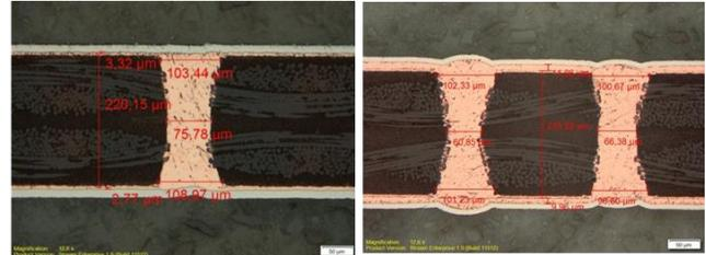
**Figure 12:** Example of optimized inclusion-free through-hole filling obtained at reduced copper thickness  $\sim 3\text{-}11 \mu\text{m}$
