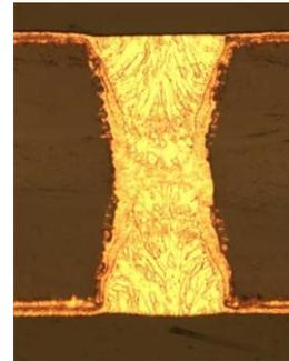
**Figure 4:** Example of filled 200µm through holes with reduced copper thickness in panel plating mode.
