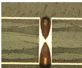
**Figure 3:** Example of X-plating in the centre of the through hole
