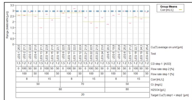
**Figure 10:** Example of metal distribution on individual unit. Behaviour of one organic additive operated in a wide working range versus different acid and chloride concentration and physical parameters.
