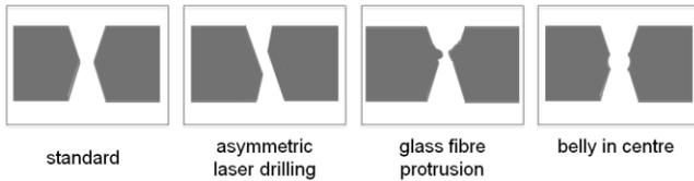
**Figure 2.** Different shapes of laser drilled through holes
