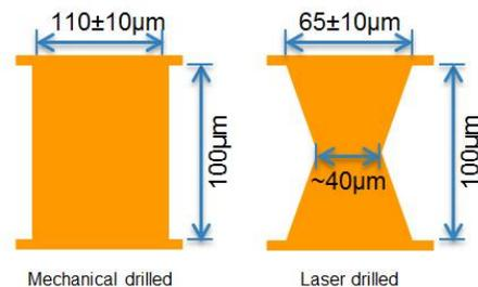
**Figure 1:** Dimensions of typical filled through holes of 100  $\mu\text{m}$  thickness
