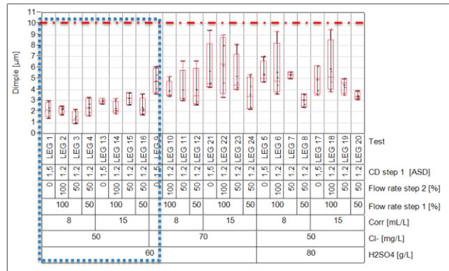
**Figure 6:** Example of filling performance on individual unit. Behaviour of one organic additive operated in a wide working range versus different acid and chloride concentration and physical parameters
