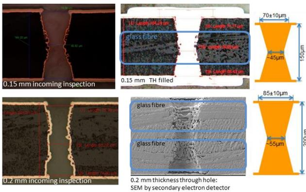
**Figure 11:** 0.15 mm thick through-hole with one centred glass fibre showing beneficial X-shape in the centre. 0.2 mm thickness through-hole with two glass fibres.
