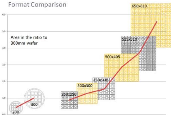
Figure 4. Area comparison of different wafer and panel formats
