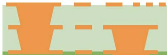
Figure 1. Schematic illustration of Cu plated features in a dual RDL package design, including  $\mu\text{Vias}$ , RDL traces and Cu pads.
