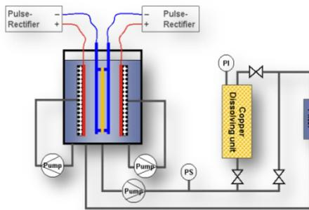
Figure 3. Plating cell fluid flow schematic of the MultiPlate® panel plating equipment
