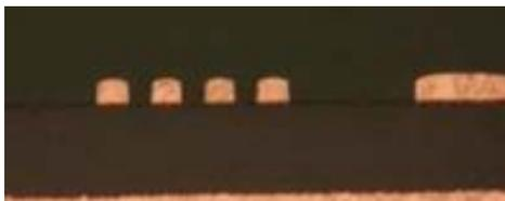
Fig. 4, Micro section of copper traces electroplated with the novel chemistry at 3ASD
