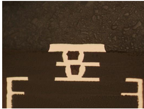
Figure 3 - Plugged and capped microvia [2]
