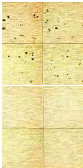
Figure 1+2: NVA test with 1,5 µm Ni/ 0.3µm Aurocor SC and post- treatments PT. Top: No post-treatment Bottom: With Betatec®
