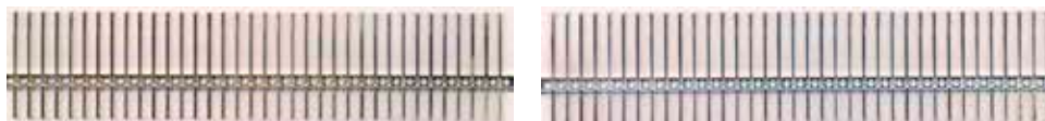
Figure 3+4: Sn Surfaces after PCT (105 °C, 85% RH and 1,2 bar). Left: without Betatec; right with Betatec®
