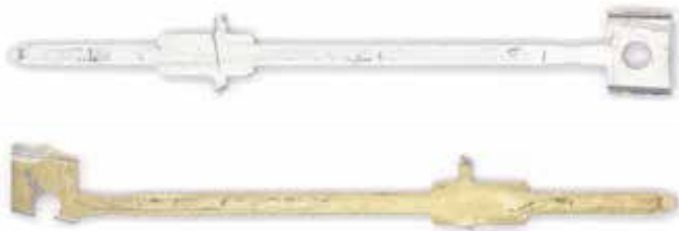
Figure 1: Connector pins treated with and without PostDip SN 260 after exposure to 260 and 285 °C
