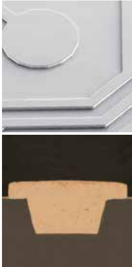
Figure 1: Plating fine lines and Cu pads Figure 2: Microvia filling CD \leq 20 \mu m
