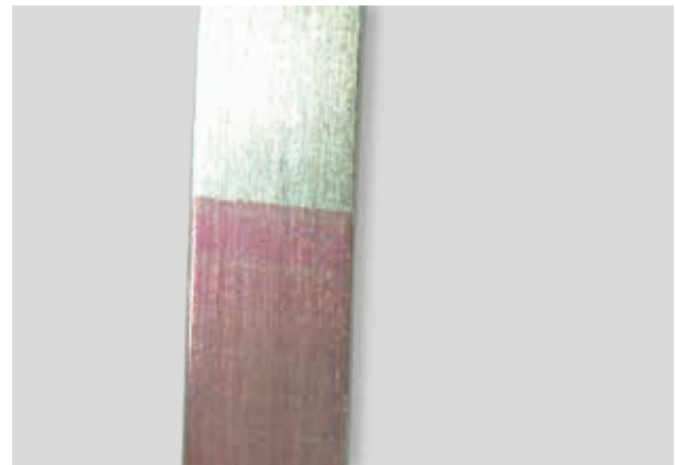
Fig. 2: Arco Test showing full wetting of the AgPrep treated silver surface (strong adhesion)
