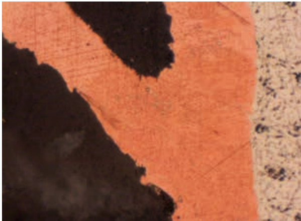
Figure 1: Cu to Cu interconnect remains intact after extreme thermal shocking
