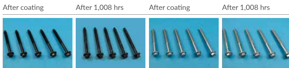
Figure 2 + 3: Surface appearance of Zinni® AL 450 + Unifix® Ni 3-30L + Corrosil® Plus 315L
