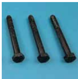
Figure 1: Surface appearance of Zinni® AL 450 + Tridur® ZnNi H1 + Corrosil® Plus 315L, after 6 cycles of corrosion test acc. to Ford L467 / Volvo ACT-II VCS 1027
