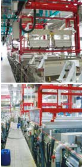
Figure 1: Barrel plating line Figure 2: Rack plating line
