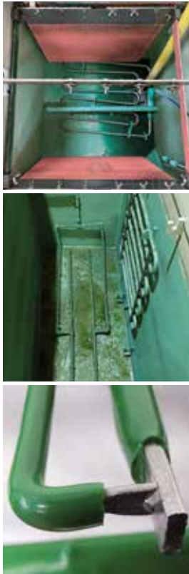
Image 1-3: Cu plate-out on cathodes Minimal sludge generation Stripped rack tip
