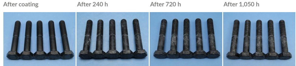
Figure 1: Surface appearance of Zinni® AL 450 / Tridur® ZnNi H5.2 / Tridur® Finish 300 after NSST (Neutral Salt Spray Test)
