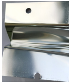
Figure 2: Sample test with LCD and low temp.: 1 ASD, 16 °C
