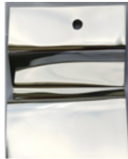
Figure 3: Sample test with HCD and high temp.: 3 ASD, 20 °C
