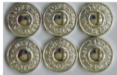
Figure 5: Sample test in barrel, 0.6 ASD, 16 °C
