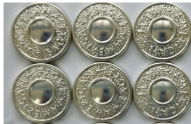
Figure 4: Sample test in barrel, 0.4 ASD, 16 °C
