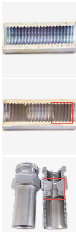
Figure 1: Zinni® AL 450 shows homogeneous thickness distribution and deep throwing power even in LCD areas inside of a sleeve (cross-cut).
