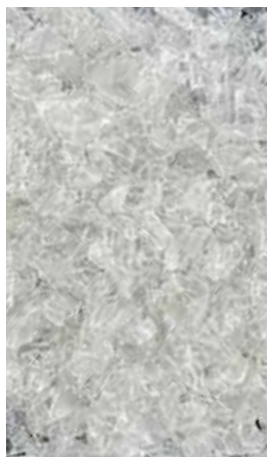
Image 1: PET flakes after conventional washing process still containing ink contamination
