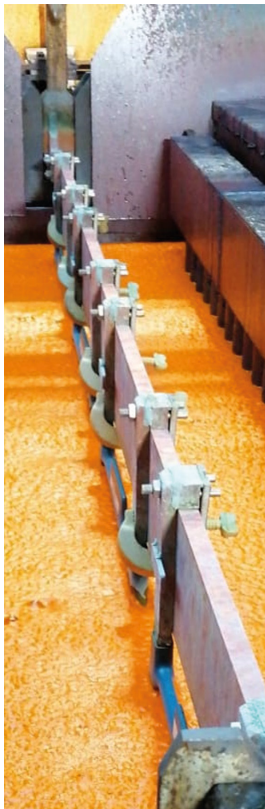
Image 1: Wetting Agent 100 foam blanket on bath surface of chrome plating bath
